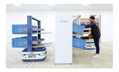
Flexytote<sup>®</sup> is the key to **versatility** : this **flexible, scalable** transport system follows optical marking on the floor and does not require complex installation, its layout can be **reconfigured as and when required.**
